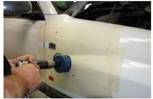
8b Using a air hack saw or similar cut a straight line between top and bottom of holes.
