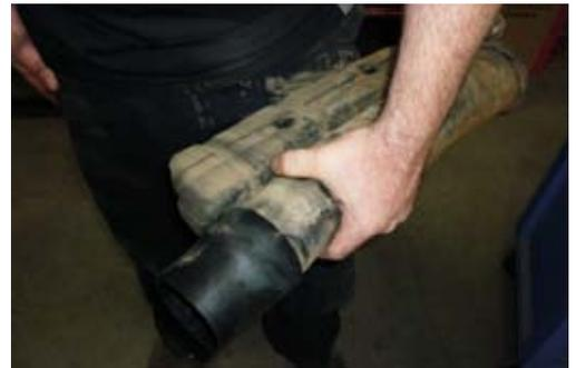
19. Remove foam seal from air box elbow under mudguard.
