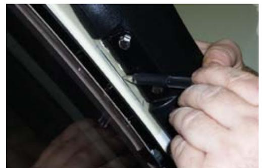
13. Remove bracket from snorkel and hold against pillar in position previously marked and mark three mounting holes. Drill holes to 7.5mm.
