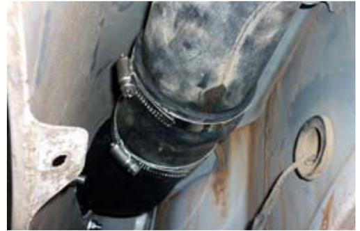
21. Check all hose connections and air box for potential leaks and seal as required.
