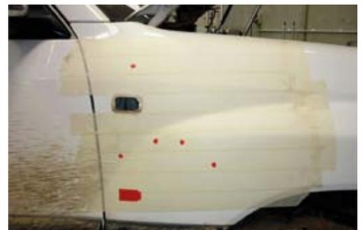
8a. Remove template. Using a 95mm hole saw cut two holes as marked
