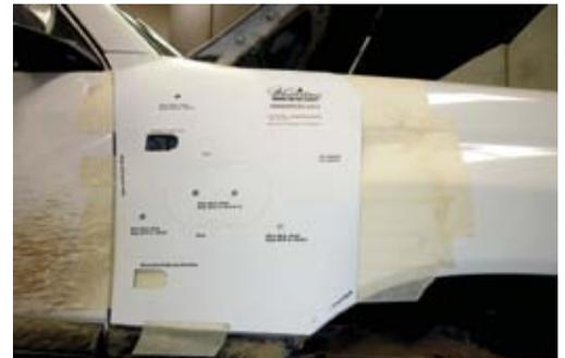
7. Using a felt tipped pen, mark all holes and new location for side indicator.
