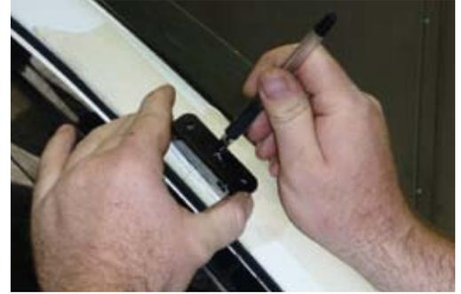
14. Apply silicone sealant to holes. Insert mounting plugs and attach mounting to pillar using self-tapping screws provided.
