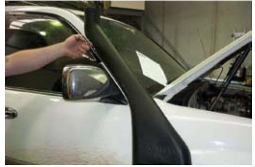
18. Attach rubber joiner to air entry duct and secure with hose clamp provided.
