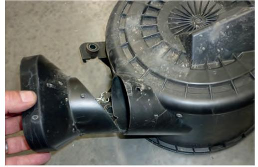
18. Position air cleaner adaptor over air cleaner intake and drill two mounting holes to 5mm.
