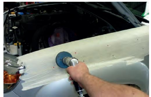
7. De-burr and rust-proof all holes (this applies to all holes drilled after this step).
