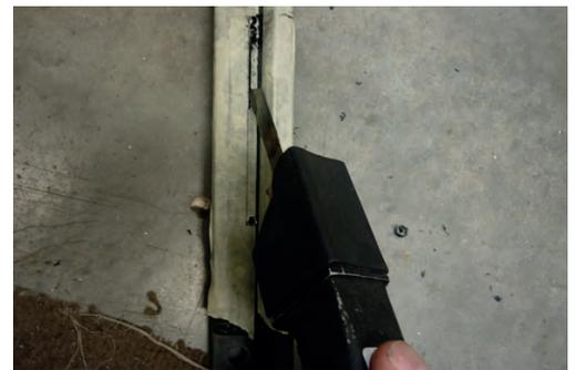
16. Refit plastic trim to pillar allowing bracket to pass through slot created in previous step (enlarge slot to clear bracket if required). Refit door rubber.
