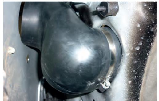
22. Attach snorkel body to mudguard using M8 Nylock nuts and Body washers, making sure snorkel outlet engages with rubber joiner and secure with hose clamp.
