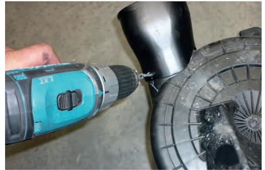
19. Seal adaptor to air cleaner intake using silicone sealant and secure in place using pop rivets provided.
