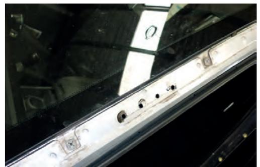
13. Apply masking tape to plastic trim removed in Step 8. Hold trim in position on pillar, mark location of pillar bracket onto plastic trim and remove trim from pillar.
